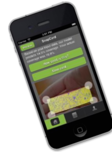
SnapCard WSP coverage measurement
