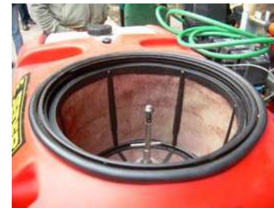
Strainers equipped with nozzles for rinsing PPP cans
