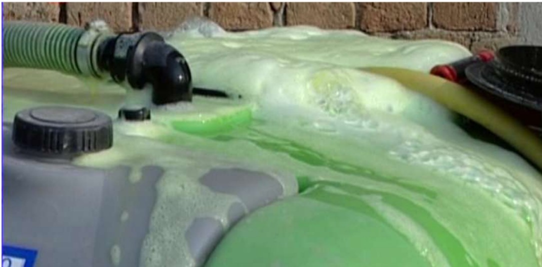
Sprayer tank overflowing
